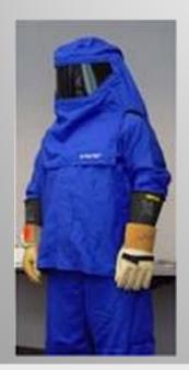
Category 4 Flash Suit in the front of the switchgear. In the rear of the switchgear, even a Cat 4 suit would not guarantee survival when standing behind the switchgear (less than 36" Working Distance).
